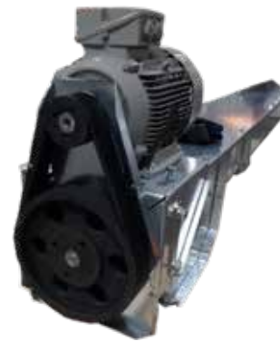
— Photo of screw conveyor head motor drive
