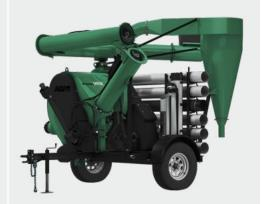
A dust collector is easy to attach and gives you flexibility to collect or direct debris.
