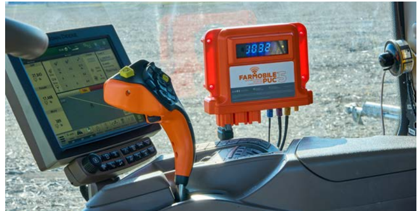
Farmobile's PUC™ is an in-cab device that captures a farm's agronomic and machine data with every tractor pass.
