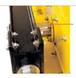
4 Heavy-duty center pull takeup frame Packing gland shaft seal
