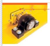
Heavy-duty long life pillow block roller bearing Packing gland shaft seal
