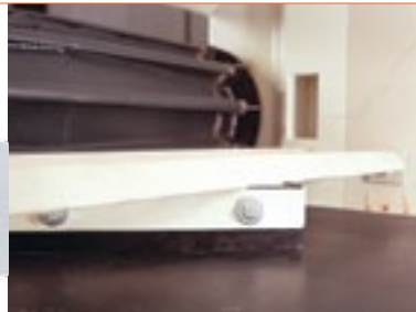
2 V-plow prior to self-cleaning, reloading tail pulley.
