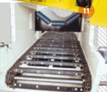
11 Internal view of reloading belt cleaner. Patent Pending (Belt not shown).
