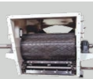
10 Head pulley showing reloading belt cleaner.
