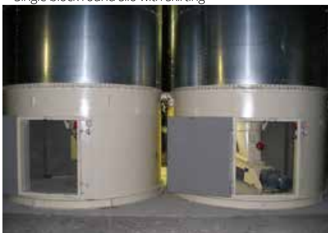
Flat-bottomed round silos with planetary extractors
